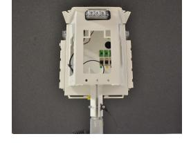
With the head unit complete, rotate it to the desired orientation. When in place, tighten and clamp the black quick release lever. Check to make sure the lever is clamped tight to prevent unit from rotating.
