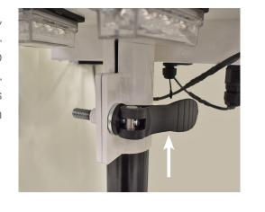
Use hand crank to raise mast until guy wire is almost tight. Allow wire to unspool as mast is raised. DO NOT overtighten. When the mast is fully raised, make sure the crank arm is positioned to the left of the mast as pictured. This allows room for the tongue to fold into place in STEP 16.
