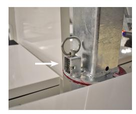
Slide the top hooks of left camera (labeled left) into the top slots of head unit (labeled left) as pictured. Insert left camera plug (red) into the slot marked with the red dot. Insert red/black wire into top green slot above it as pictured. Lower camera into place and tighten black knob.
