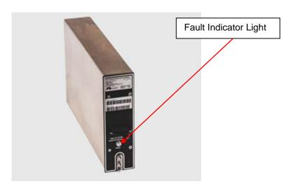
The fault indicator light is not an indication of available battery capacity. Battery capacity can only be verified by test or replacement of the battery pack. The DBC was designed to meet the operational energy storage requirements when the following conditions are met IAW the DBC CMM 24-31-05, Rev 7
