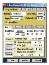
Speed-based deactivation is a critical tool when more than one detection channel is programmed to extend green. For example, when a queue reduction channels is used in combination with an advance detection channel, speed-deactivation of the queue reduction channel will ensure that the advance detection can terminate the phase as soon as the first safe gap in traffic is found.
