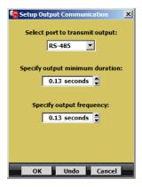
The figure above shows the settings for communicating to a Click 172/174 rack card. The minimum duration of each contact closure is 130 ms and all standard traffic controllers should be capable of counting these pulses. When receiving data from SmartSensor Advance, the Click 172/174 racks cards should always be configured in Actuation mode.
