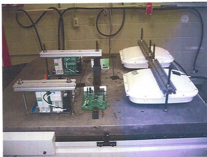
WAVETRONIX SmartSensor Matrix equipment, configured for Vibration and Shock testing in X, Y & Z orientations.
