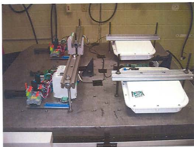
WAVETRONIX SmartSensor Matrix equipment, configured for Vibration and Shock testing in X, Y & Z orientations.
