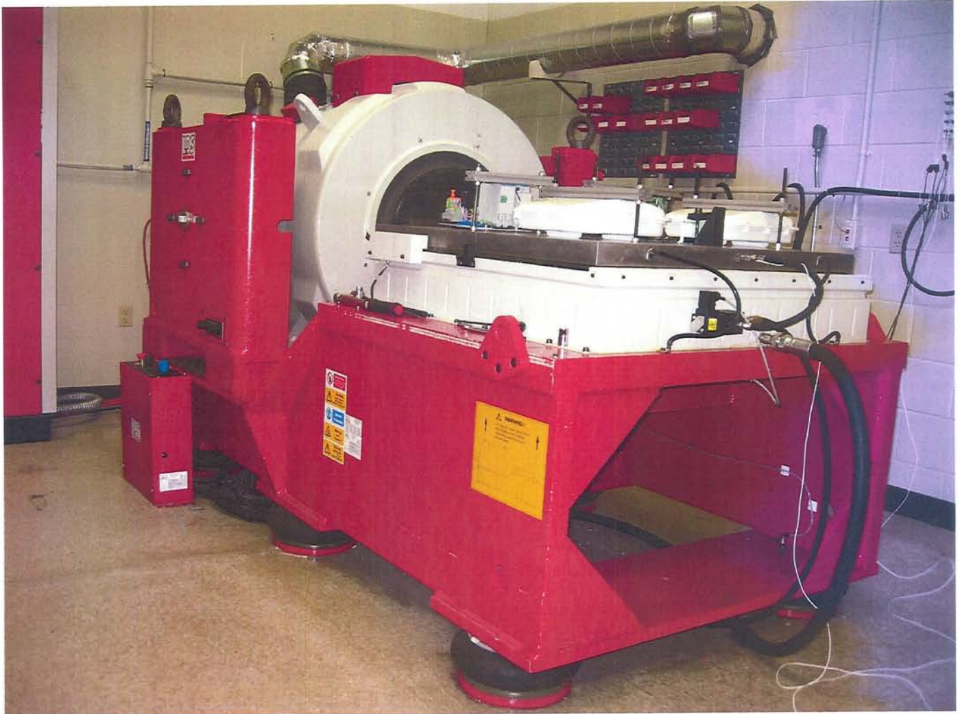
WAVETRONIX mounted to LDS V8-440 Vibration Simulation System.
