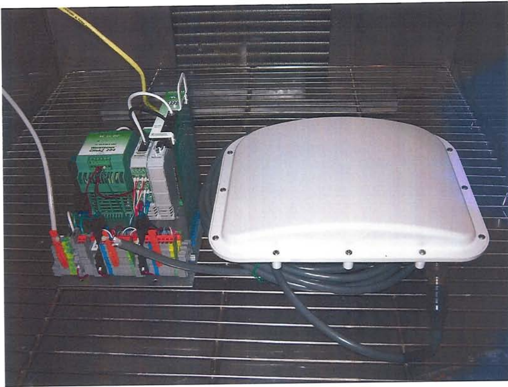
WAVETRONIX SmartSensor Matrix equipment configured for Temperature /Humidity.
