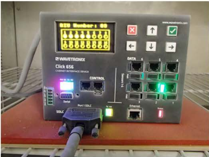
WAVETRONIX Click 656 - Configured for Temperature /Humidity Testing. (NOTE: LCD Display remains legible operating at Cold or Hot extremes.)
