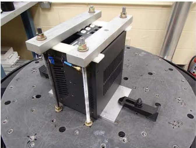
WAVETRONIX Click 656 – Configured for Vibration and Shock Testing in X, Y & Z axis orientations.
