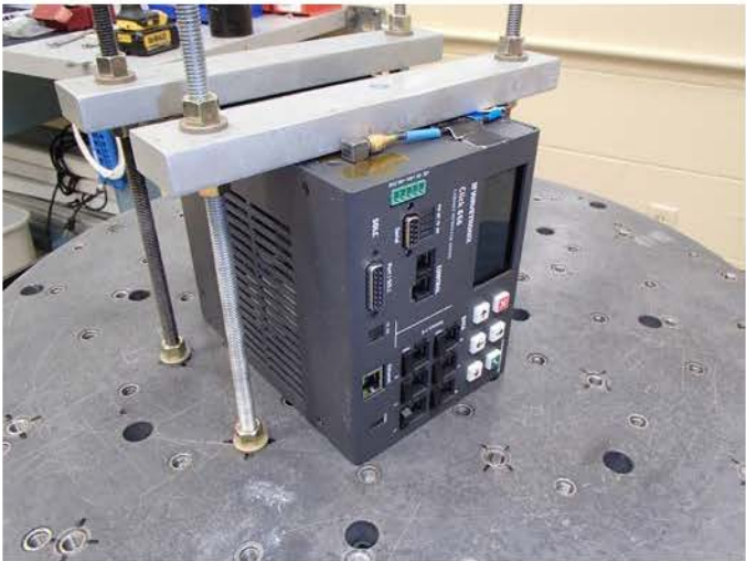
WAVETRONIX Click 656 – Configured for Vibration and Shock Testing in X, Y & Z axis orientations.
