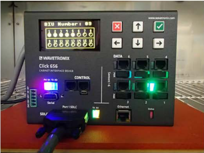
WAVETRONIX Click 656 - Configured for Temperature /Humidity Testing. (NOTE: LCD Display remains legible operating at Cold or Hot extremes.)
