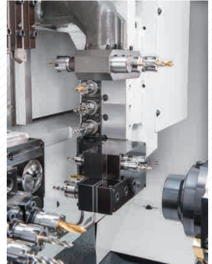
Expansion Cross live tool x 3 Front-end live tool x 5 Rear-end live tool x 2
