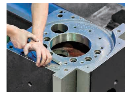
Hand scrape on spindle and spindle motor contact surfaces of headstock.
