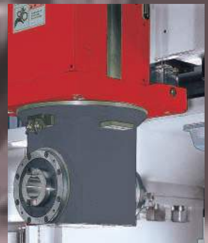
Horizontal head structure
