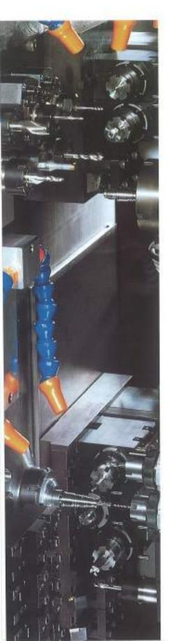
An increased productivity thanks to its two oppossed slides. The subspindle enables all rear side machining.
