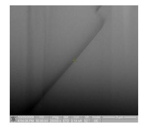
Figure 4 SEM cross-section of the silicon cell across propagated crack, image size is 9.5 x 11 microns. Figure 3 SAM image of 3.6 x 3.6 mm map with submillimeter pinhole. Note that unopened cross cracks provide cleavage directions when the cell is broken.
