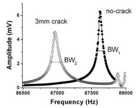
Figure 1 Deviations of peak parameters caused by a crack.
