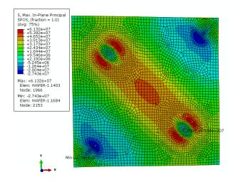
Figure 5 FEA calculation of stress profile under 5 mm wafer deflection using proposed AS procedure (front surface). Maximum stress of 61.3MPa is in the contact regions of suction cups and wafer.
