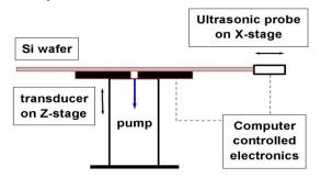
Figure 2 RUV system schematic
