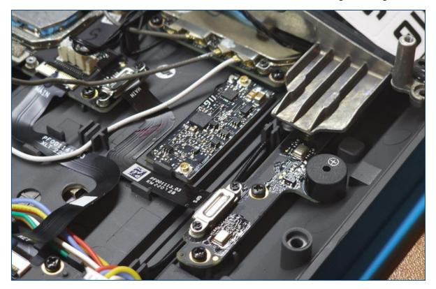
Figure 1: DJI911 NeoBooster hardware modification soldered into the DJI RC PLUS controller
