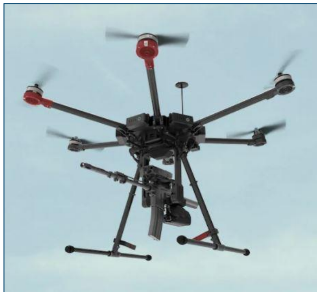
Figure 13: Assault rifle attached onto a DJI Matrice 600 by SMASH SHOOTER
