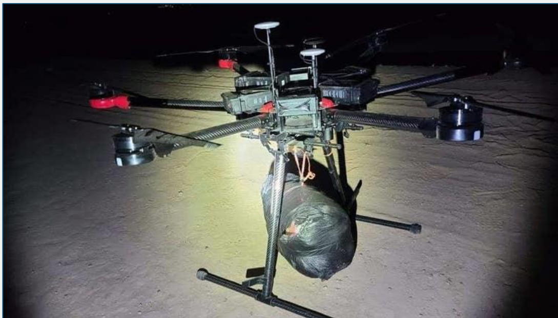
Figure 7: The heavy-lift drone seized, likely a DJI Matrice 600 Pro with payload dropping mechanism
