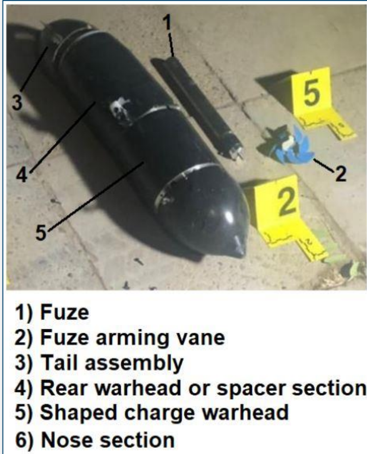
Figure 6: Breakdown of the components of the bomb - https://twitter.com/blueboy1969/status/1457479574758076417
