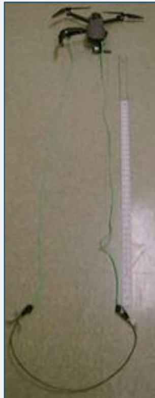
Figure 1: Incident DJI Mavic 2 used to disrupt substation
