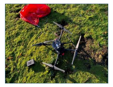
M300 drone crash was due to excessive vibration of parachute system not securely attached <a href="https://www.gov.uk/aaib-reports/aaib-investigation-to-dji-matrice-200-v1-uas-registration-n-slash-a-210919">https://www.gov.uk/aaib-reports/aaib-investigation-to-dji-matrice-200-v1-uas-registration-n-slash-a-210919</a>
