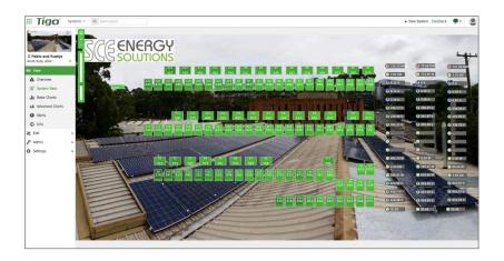
**Tigo Energy Intelligence** enables SCE Energy Solutions to view site performance down to each individual module (left). In addition, SCE and customers view the incremental energy production enabled by Tigo optimizers, shown in the stacked green bars (right).
