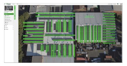
**Tigo Energy Intelligence** enables SCE Energy Solutions to view site performance down to each individual module (top). In addition, SCE and customers view the incremental energy production enabled by Tigo optimizers, shown in the stacked green bars (bottom).
