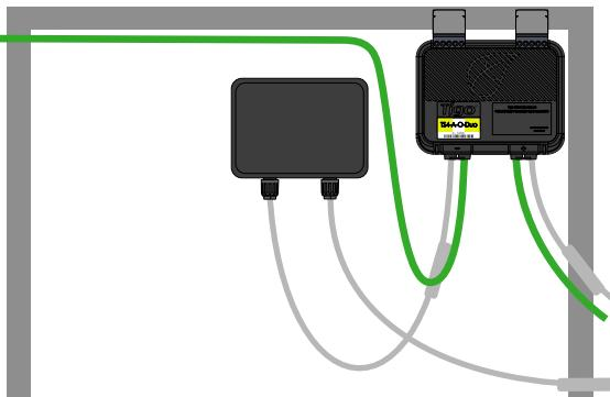
Note: When installing TS4-A or TS4-A-Duo, connect the input cables to the PV module before connecting the TS4-A output cables in series.
