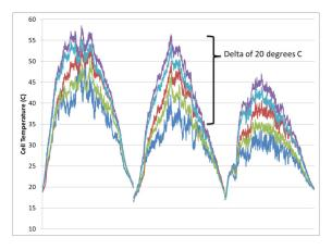
Figure 4: Cell Temperatures on Commercial Rooftop
