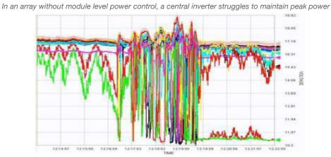
Figure 7: Module Voltage Patterns During Transient Cloud Cover
