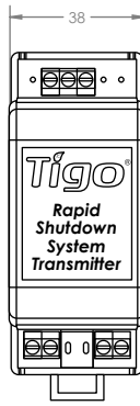
RSS Transmitter - Front View
