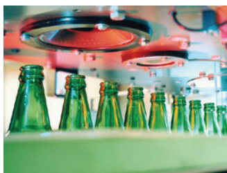
View of a row of an empty bottle inspection system, which uses pixelfly cameras for the improved resolution inspection (IRIS), courtesy of Krones AG, Neutraubling, Germany
