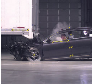
Full scale crash test of a car hitting the rear end of a truck for deformation analysis in order to develop safer vehicles.
