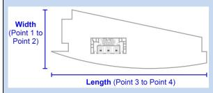
Figure 3 Length and width of the pictorial representation of a floor for an unusual floor shape
