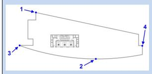
Figure 2 Identifying outer-most points of the pictorial representation of a floor for an unusual floor shape
