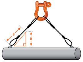
Note: When using 3 or 4 leg slings, it is possible that only 2 of the legs may see loading. Therefore, it is common practice to calculate tensions using only 2 legs to be sure no overload occurs.
