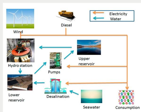
Figure 1: Schematic view of the wind-hydro system of El Hierro showing the flows of electricity and water
