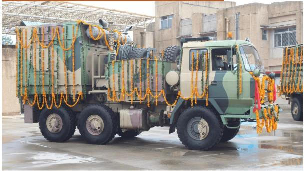
The Indian Army has inducted a lighter and compact version of indigenously developed Weapon Locating Radar (WLR) called Swathi Mountains. Developed by Bharat Electronics Limited, Bengaluru, it is an advanced, electronically scanned phased array radar, specifically designed for operations in mountainous and high-altitude areas.
