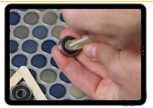
2. Use included WOODEN DOWEL to help poke tube through middle of bearing
