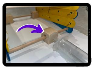
GLUE THE BOTTOM END OF A SYRRINGE ONTO THE CUBE
