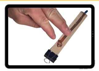
Place Copper tape on this side, and MAKE A PILE with extra tape on the dot you drew.
