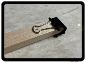
FLIP STICK OVER...drop metal hammer and make a little dot in middle of the loop.
