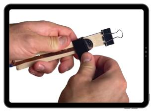
Put a little bit of tape onto the battery to hold it in place!
