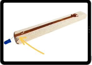
On side with <u>LONGER LED WIRE</u>, Place COPPER TAPE along middle \*\*Tape must cover/start at LED wire
