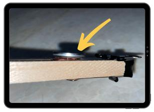
Place battery on top of tape with the NEGATIVE SIDE DOWN!!
