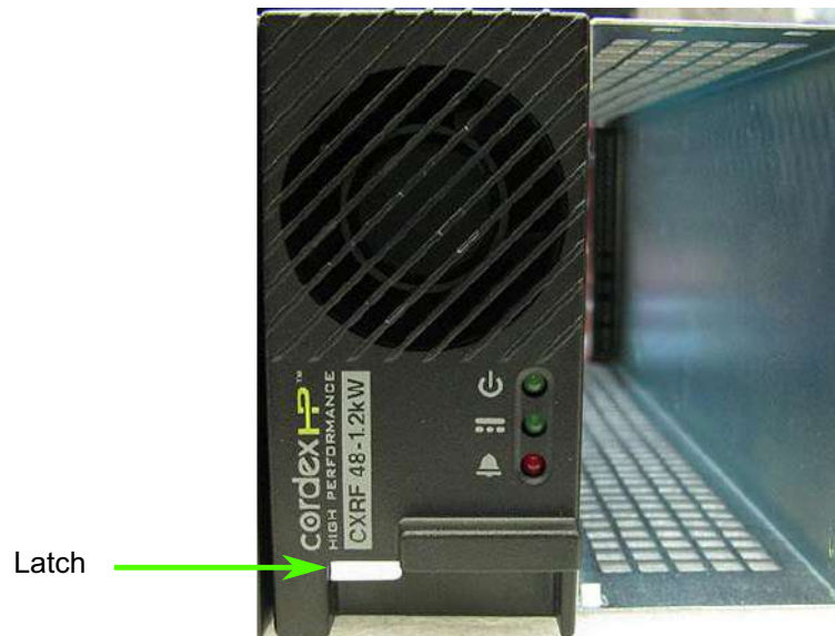
Figure 14: Removing a Rectifier from the Shelf
