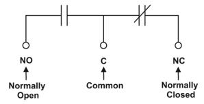
Relays can be programmed to energize or de-energize during an alarm condition (see controller software manual). When the controller reset button is pressed or power is lost, all relays de-energize.
