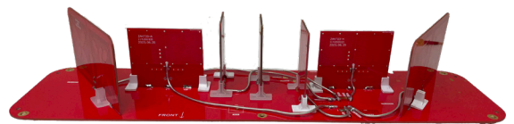
High-performance cellular (LTE) and Wi-Fi antennas controlled by ZetiLink™ switching technology
