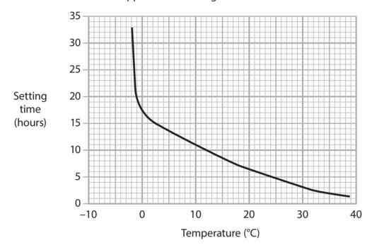
Matt needs to advise a customer about concrete setting time. He uses the graph to explain how the temperature affects the time it takes for concrete to set.
