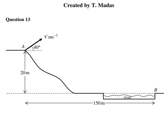
A golf ball is struck from a point A with a speed  $V \text{ ms}^{-1}$  at an angle of elevation 40°, so it can clear a river. The ball is modelled as a particle moving freely under the action of its weight. In order to clear the river the ball must land further than a point B on the opposite river bank. The point B lies a vertical distance of 20 m below the level of A and a horizontal distance of 150 m from A, as shown in the figure above.
