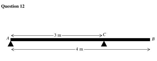
A plank of wood AB has length 4 m and mass 40 kg. The plank is smoothly supported at A and at C, where AC = 3 m, as shown in the figure above.
