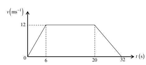
The figure above shows the speed time graph (t,v) of a car travelling along a straight horizontal road between two sets of traffic lights.
