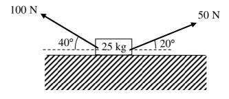
The figure above shows a small box of mass 25 kg, pulled by two light inextensible strings along rough horizontal ground.
