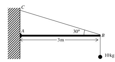
The figure above shows a uniform rod AB, of length 3 metres and of mass 20 kg, smoothly hinged at the point A, which lies on a vertical wall.
