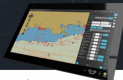
The SEALL ECDIS is one of the first marine software systems to include a multi-touch screen interface, changing the way it's operated and making it one of the simplest ECDIS systems to operate on the market.
