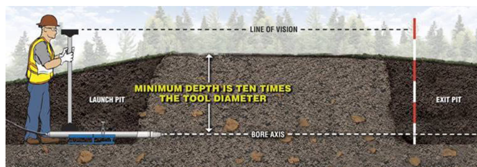
Figure ES.6.2: Two Pits, with Ground Between Undisturbed, Used in Trenchless Service Line Installation
