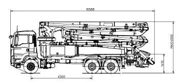
Dimensions varying according to truck assembly
