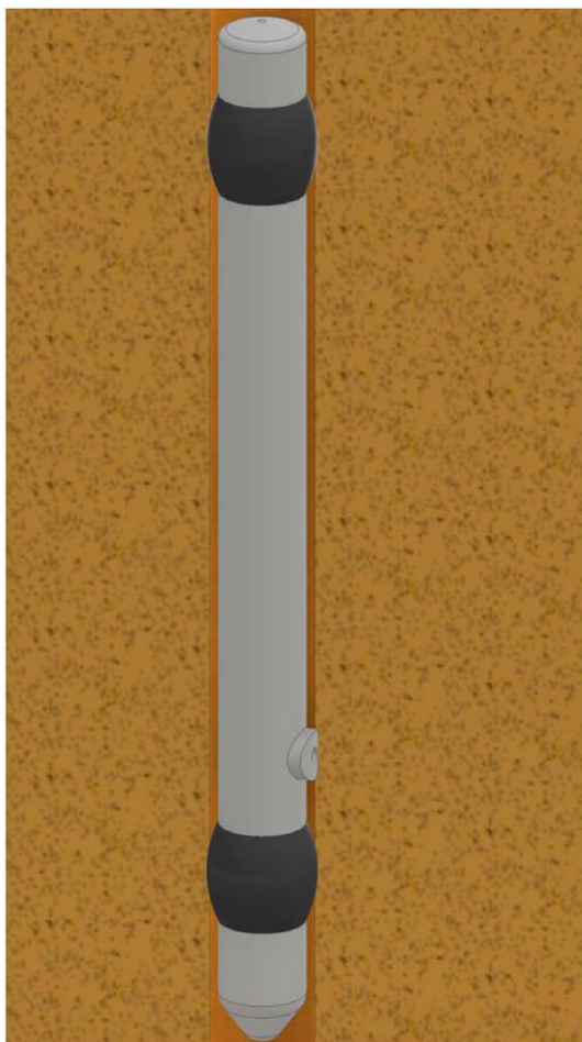
Figure 10—The tool has been lowered into the well, and the packers have locked it in position.
