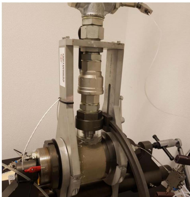
Figure 5—A picture of a 4" Berea core during drainage with transparent Isopar H oil in the chamber. Probe coming in vertically from the top.
