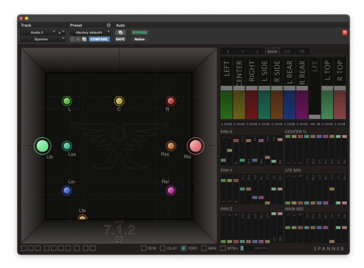
The pucks in the "Panfield" represent input channels and for each there are a set of faders which control the specific parameters which determine how that input channel is treated.
