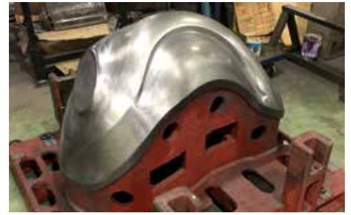
This example is the fender of a VW Beetle. The male and top hat pieces are shown here. Notice the top hat lip.
