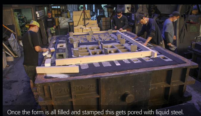
Once the form is all filled and stamped this gets pored with liquid steel.
