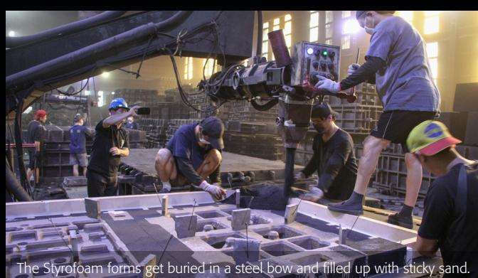
The Styrofoam forms get buried in a steel bow and filled up with sticky sand.
