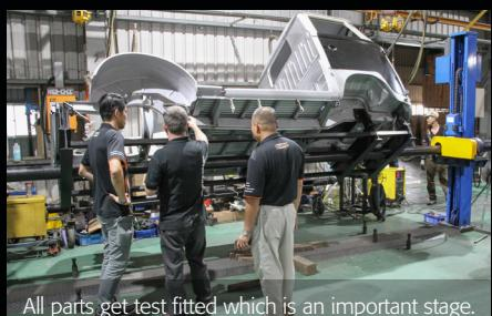
All parts get test fitted which is an important stage.
