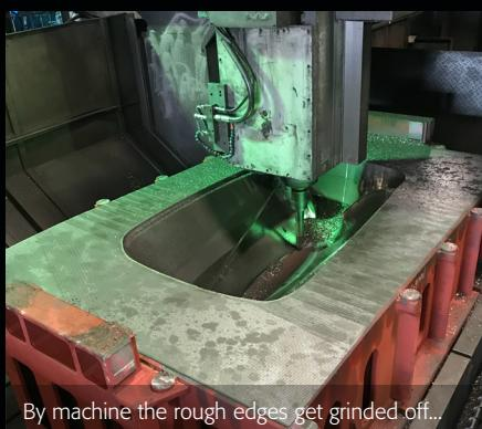
By machine the rough edges get grinded off...
