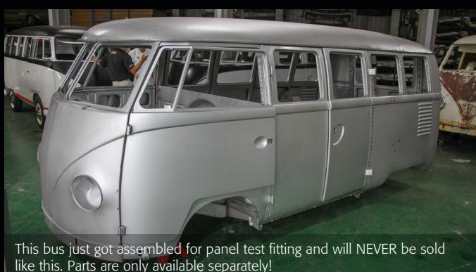
This bus just got assembled for panel test fitting and will NEVER be sold like this. Parts are only available separately!
