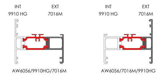
Where customers require profiles in the reverse position, should indicate by use of drawings when placing their order. Where no guidance is provided, AluK will always supply as per the above as presented in the AluK Technical Manual.
