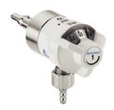
The DPG 2 flowmeter with pre-adjusted flows is used to set the flow of a gas that is to be delivered to pa-tients through the respiratory tract. It should be connected to a source of pressured gas on the wall either using a direct probe or a rail mounting system. It must be fitted at its outlet either with a humidifier/nebulizer or with an outlet tubing nipple.
