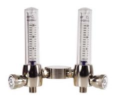
The dual flowmeter splitter adapter can be used to connect two flowmeters to one single supply point and supply medical gas to two patients simultaneously. It can be connected to the gas distribution system using suitable AFNOR NF S 90-116, DIN 13260-1, UNI 9507, BS 5682 compliant probes or probes with a G1/4" M R thread. The two flowmeters are connected to the body of the dual splitter adapter by a M12 x 1 - G 1/4" nipple.
