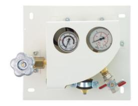
Third source panel consisting of a single reducer EURO/A model, two pressure gauges, a High Pressure shut-off valve, gas specific inlet connection, a Ø10 mm weld-on pipe connector on the outlet; its maximum capacity in Nitrogen at 7,5 bar outlet pressure is 48 Nm³ / h, 800 Nl / min.
