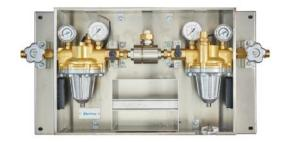
Single stage fully automatic control panel for high-flow medical gases: composed of two GIGANT/R, two High Pressure shut-off valves and two Low Pressure shutoff valves for maintenance, stainless steel case, specific gas inlet connection, in output it has a  $\emptyset$  22 mm weld-on pipe connector; the maximum flow rate in Nitrogen at 9 bar pressure is 150 Nm³ / h, 2500 Nl / min.
