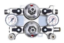
The 2nd stage unit is made of cast CW614N chemically nickel-plated brass; the device has a pressure gauge that shows the pressure upstream of the reducers and another pressure gauge that shows the operating pressure; there is also a G 1/4" F R threaded fitting which can be used to install any kind of accessory.
