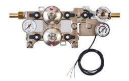
The unit is made of two chemically nickel-plated brass castings, one casting for the regulators bodies, and the other casting for the zone shut-off valve; the regulator body has two decompression lines with two EURO/A regulators connected in by-pass through four ball valves, two on the inlet and two on the outlet of the same.
