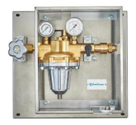
Fourth source panel consisting of a single GIGANT/R reducer, two pressure gauges, a High Pressure shut-off valve, a gas specific inlet connection and on the outlet a  $\varnothing$  22 mm weld-on pipe connector. The maximum flow rate in Nitrogen at 9 bar pressure is 150 Nm³ / h, 2200 Nl / min.
