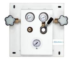
Control panel for medical gases, with automatic exchange and manual reset; composed of two lines of EURO regulators, complete with High Pressure contact pressure gauge, High Pressure shut-off valve, two overpressure discharge valves, incorporated in the reducers, with  $\varnothing$  12 mm weld-on pipe connector and a Low Pressure shut-off valve for the maintenance
