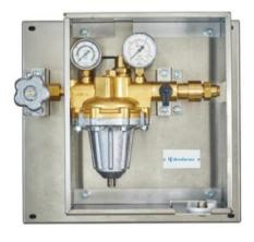
Third source panel consisting of a single reducer, two pressure gauges, a High Pressure shut-off valve, a gas specific inlet connection and on the outlet a  $\varnothing$  22 mm weld-on pipe connector; the maximum flow rate in Nitrogen at 7,5 bar pressure is 120 Nm³ / h, 2000 Nl / min.
