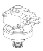
The stainless steel low pressure switch is designed to protect devices for the compressor and refrigeration circuit. Monitors the refrigeration system for a loss of refrigerant charge, and may also be helpful in stopping the evaporator (indoor) coil from freezing up due to a dirty filter or low airflow over the coil.
