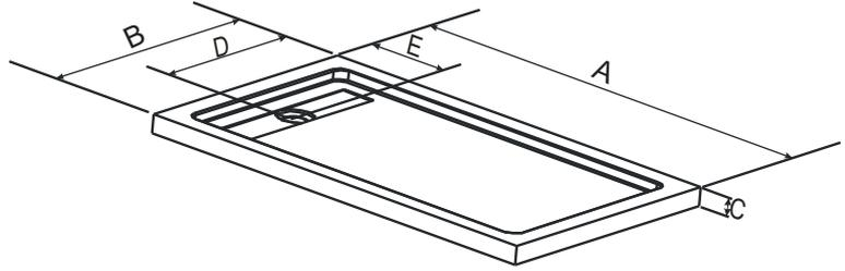
\*Tolerance on dimensions:  $\pm 1/4"$  [6mm]
