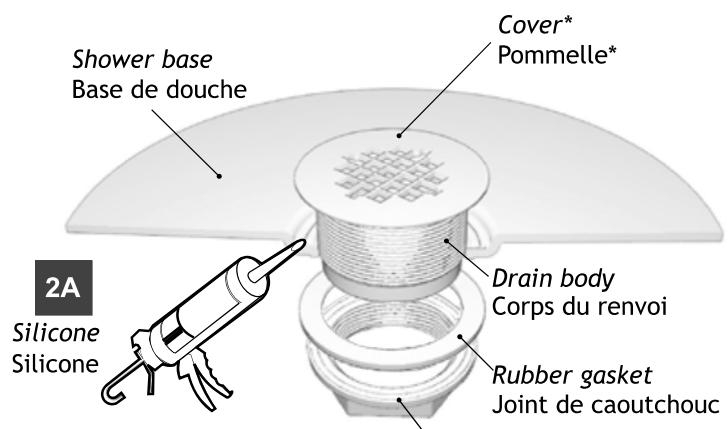
Components might vary according to the model of drain used.
