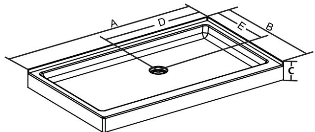
\*Tolerance on dimensions: ±1/4"[6mm]
