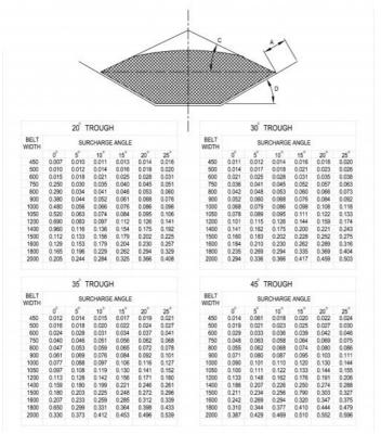
THE TABLE GIVEN ON THE PRECEDING PAGE CAN BE USED AS FOLLOWS: \*A\* TO FIND TONNES/HOUR T/Hr = 3.6XBELT SPEED (M/SEC) X CSA (M ) X MATERIAL DENSITY (Kg/M )
