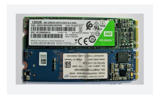
The Western Digital SSD (green) in the previous photograph uses SATA/AHCI. The Intel SSD (blue) on the other hand uses NVMe. The NVMe SSD cannot be connected to a computer with a regular SATA adapter or write-blocker. Despite the fact that both cards have the same B+M key M.2 physical interface, their electrical interfaces and command sets are completely different.
