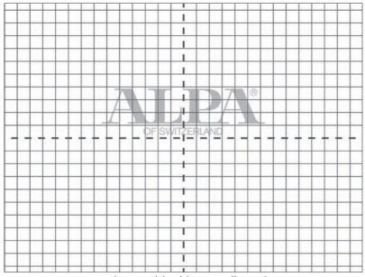
grey: base grid with zero distortion real image circle at 150% size spacing of the grid lines 2 mm (@ 100%)
