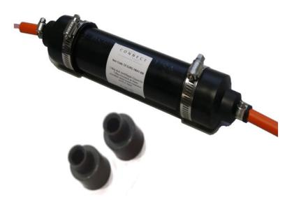
The 1-Way duct-microduct joint/repair closure consists of piece of duct shaped body and two flexible reducing duct couplers. The couplers are secured onto the body and the duct with the included cable straps. Included in the kit is the bonding hardware to allow for tracer wire continuity.
